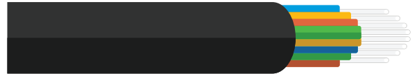
Fiber-optic cables are made of fragile glass, so they're protected by many layers of a kevlar-like material to keep them from breaking.
